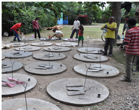
Photo Credit: iDE (International Development Enterprises). The photo depicts iDE-trained businesses manufacturing and curing latrine slabs.
